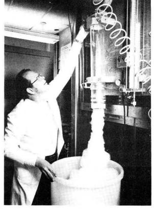
FOAM FLOWS from Pete Rand's generator in a test of the stability of aqueous foams for use as a deterrent in a high-security area.
